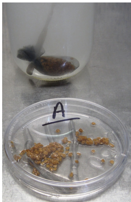
Figure 6. Nylon seed bag in HCl treatment solution, and treated seed in foreground (Exp. 31A).
