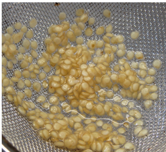
Figure 19. Appearance of seed treated with 4702 mg/L chlorine at pH 10.3 for 60 min.
