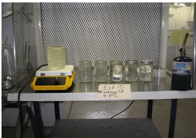
Figure 3. Set-up for chlorine disinfection experiments in laminar flow cabinet showing the seed treatment beaker on the magnetic stirrer, and the rinsing and neutralization containers.
