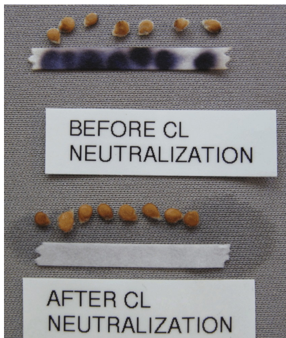
Figure 11. Effect of treated seed on chlorine residue paper before drying. Seed was placed on paper and then moved to show the purple color indicating a strong chlorine residue.
